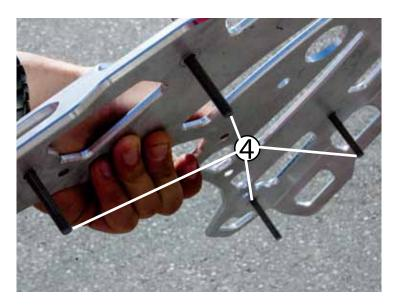
Put the (4) M6 x 45 flat head fasteners in the AltRider Rack and put it on the OEM rack, lining up the fasteners with the spacers.
