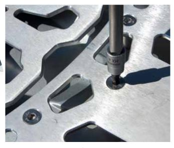
Insert the (3) M6 x 40 fasteners using a 4 mm allen tool get the fastners started and leave them loose.
