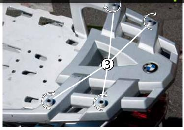
Place the M6 spacers as shown on the OEM plastic rack. Be sure to place them so that the angle-cut side is down. As best you can, rotate them so that the tops are all planar.
