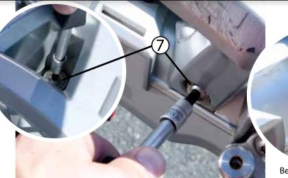
Using a T-30 torx tool, remove the (2) side fasteners and the (1) center fastener that hold the OEM rack in place. Remove the OEM rack. You will reuse the (2) side fasteners, but not the center fasteners or spacers.
