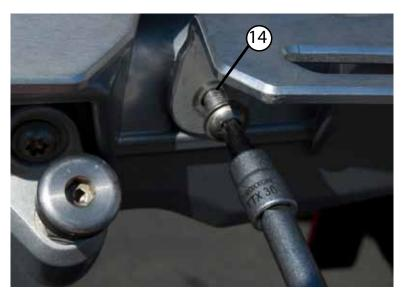
Using a T-30 torx tool, tighten the two side fasteners all the way down.
