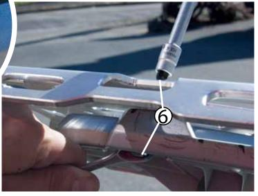
Once you are sure that all spacers are lined up properly, move on to tightening. Using a 10mm wrench and a 4mm allen tool, tighten all 4 fasteners all the way down -- not too tight, or the plastic will break.
