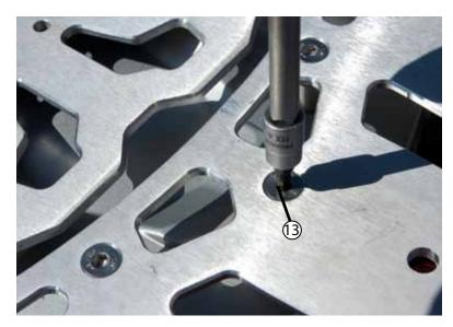
Tighten down the (3) M6 x 40 fasteners using a 4mm allen tool.
