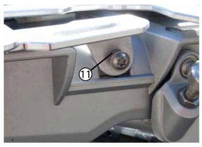
Re-insert the (2) OEM T-30 torx fasteners in either side and get them started, do not tighten these all the way down yet. DO NOT forget the OEM spacers behind the bracket.
