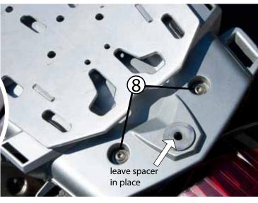
Using a T-30 torx tool, remove the (2) OEM fasteners from the plastic tail platform. Ensure that the large aluminum spacer is still in place.
